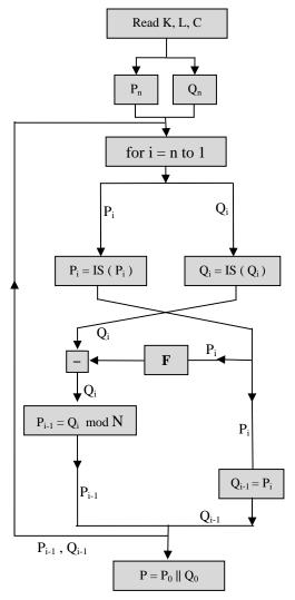
Fig 2. The process of Decryption
